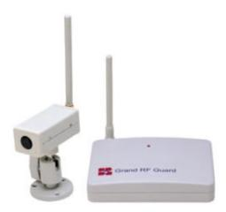
**Grand RF-Guard** includes a wireless CCD transmitter and receiver. It delivers clear CCD images and audio up to 100 meters in open area (30meters through walls or floors). Four selectable transmitting channels provides the ability to use up to four cameras simultaneously in a single area.
